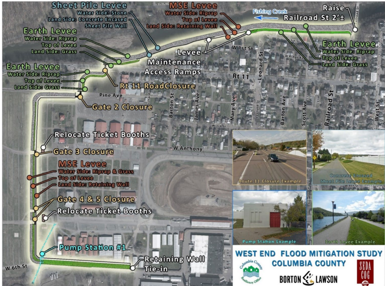
Figure 6.1 – Proposed Conditions Levee Alignment
